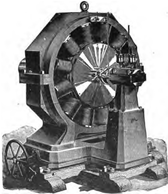
FIG. 16.—ALTERNATING-CURRENT SEPARATELY-EXCITED 12-POLE GENERATOR.
